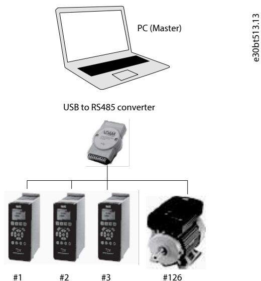
Figure 1: Connect up to 126 Nodes with a Repeater and up to 31 Nodes without a Repeater
