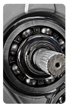
↑ Integrated g-peak sensors detect early bearing wear by measuring vibration levels, helping you take timely action before costly damage occurs. The same sensor also supports cavitation detection and speed control in pump applications.
