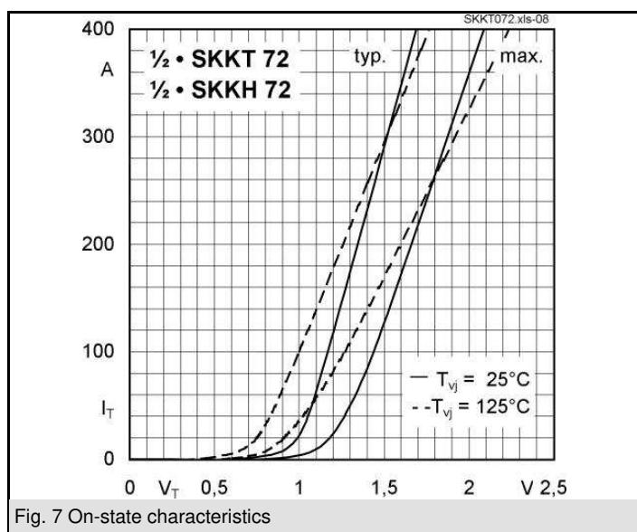
Fig. 7 On-state characteristics
