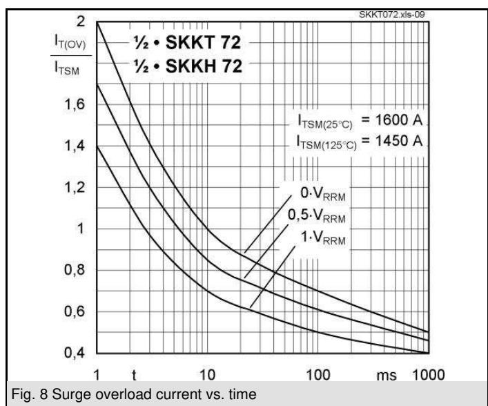
Fig. 8 Surge overload current vs. time
