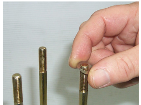
Install shims between each section
