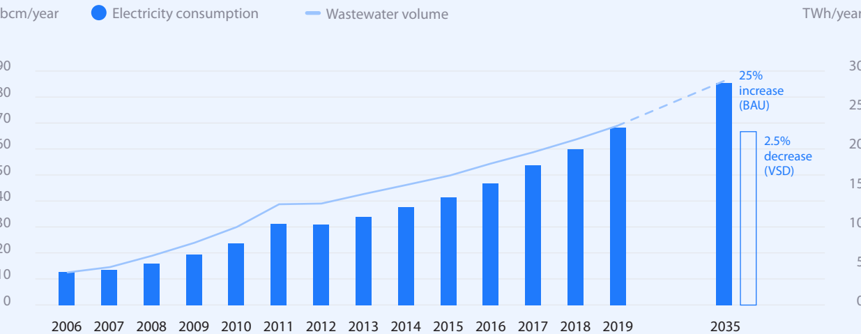
Figure 9 Wastewater volume and electricity consumption in China from 2006-2019, 121, 122 and projected wastewater volume and electricity consumption by 2035 in a business-as-usual (BAU) scenario and an Energy efficiency through VSDs scenario. In the VSD scenario, the existing WWTPs are retrofitted with VSDs, while all new WWTPs are VSD-enabled from the outset.
