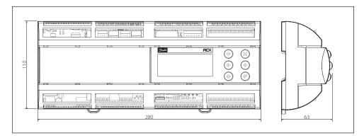
The MCX-RTU must be mounted in a space that meets the environmental standards named in the specification section of this document.
