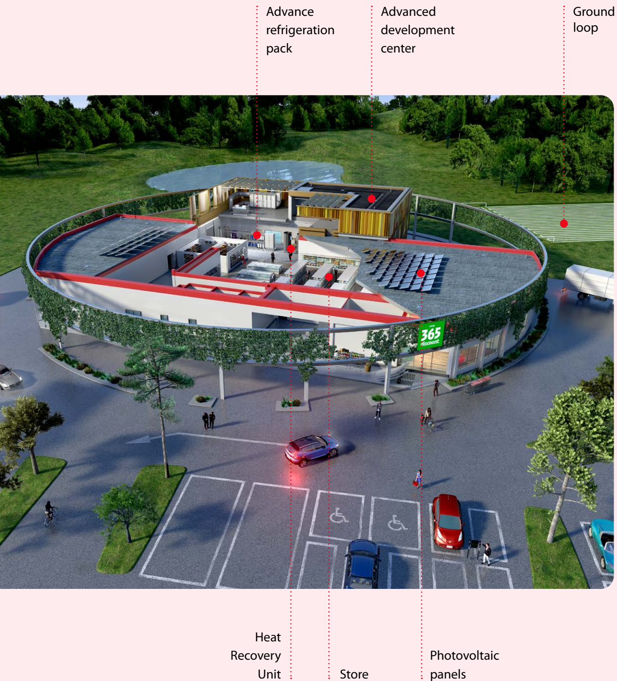
← Figure 1: Danfoss Smart Store layout with store and ADC
