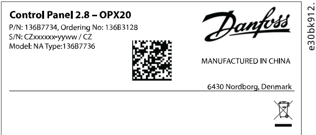
Figure 64: Example of a Control Panel Label
