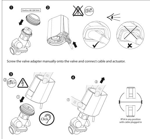
Place the actuator vertically on the valve adapter. The actuator snaps onto the valve adapter with a "click" when pressed down vertically by hand. Do not apply power until the actuator is mounted on the valve.
