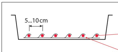
The ECfast is fixed by means of hotmelt, silicone, etc., but the best decision would be by screws or rivets.
