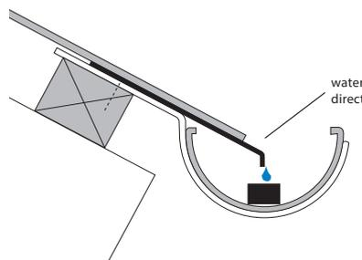
Steep roofs facing south may be exposed to the strong sunlight and as a result fast water dry out. In such cases it may be required to install some additional means to direct water towards a moisture detecting sensor.
