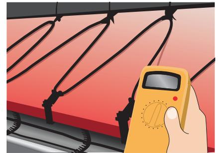
5. Install the cable(s) on the roof, in gutters and downpipes. Check once again and compare the insulation resistance and Ohm rating for constant wattage cables.
