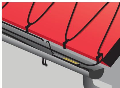
7. Extend sensor cables, cold tails/terminate cables and place connections dry. Seal all penetrations, e.g. through roofs and walls.
