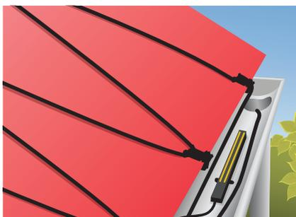
6. Install ECtemp 850 external sensor, if any, in the gutter according to the sensor manual.
