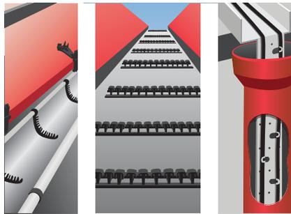
4. Install the connection box and fixing accessories in the gutters, gutter valleys, on the roof and/or the cable.
