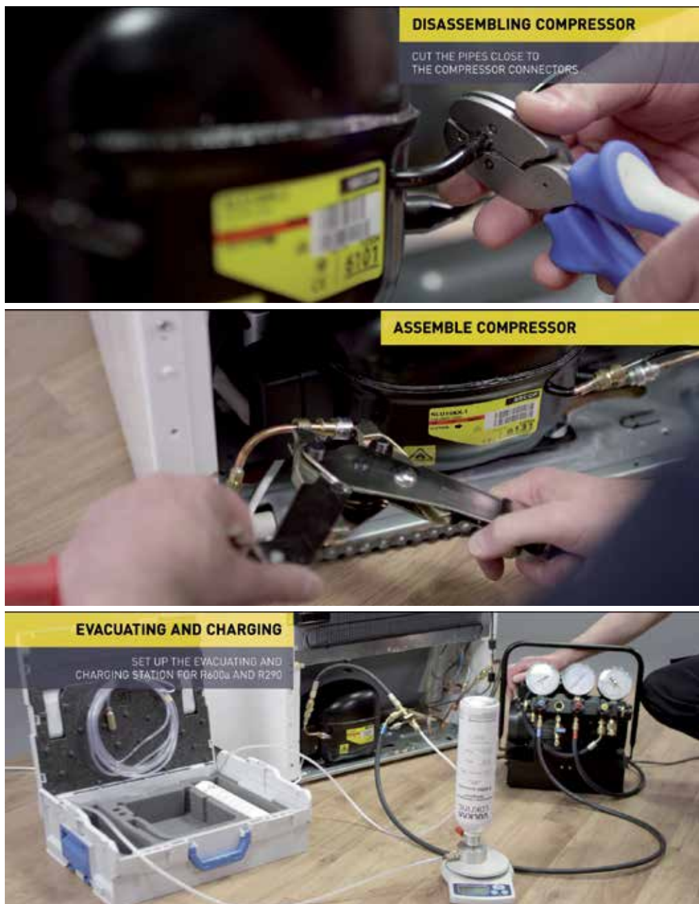
Images 5-7: Screenshots from educational film “Compressor Service for R600a/R290 - Step by Step”
