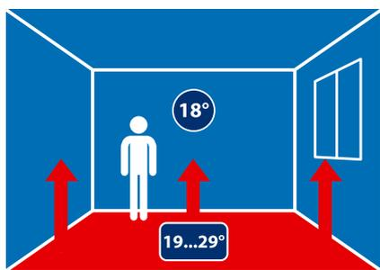
Special Danfoss thermostats are used where setting of the maximum floor temperature is necessary or advisable:
