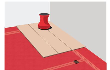
8. Make sure that the ECdry is heating before installing the floor finish. Tape the elements together. Install the floor finish directly onto the ECdry elements.
