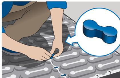
4. Install the Reflect insulated plates (EFCI Dry) on the heated areas and optionally 13 mm plasterboards on the non-heated areas. Connect the plates together with provided connection material.
