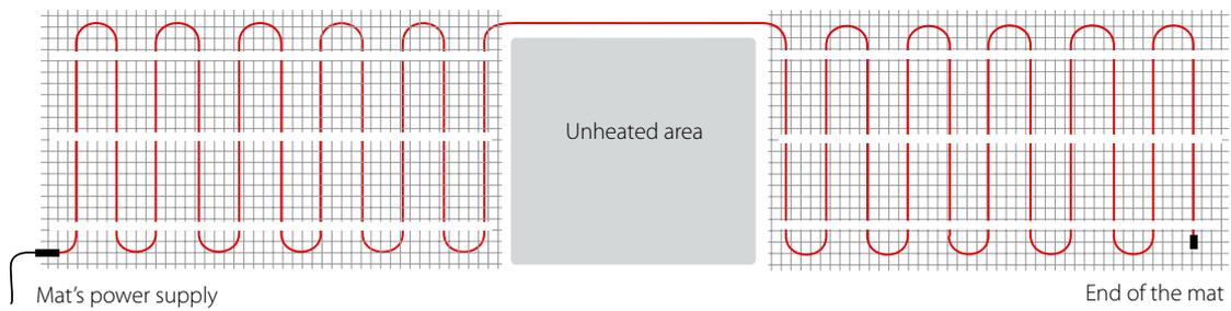
Fig. 8. Layout for a mat around an unheated area / obstacle.
