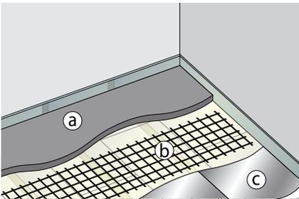
4. Install separating layer, e.g. concrete (a), metal mesh (b) or aluminum foil (c).
