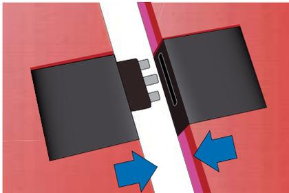
3. Remove the end stops from connectors. Put the male and female connector together by hand.
