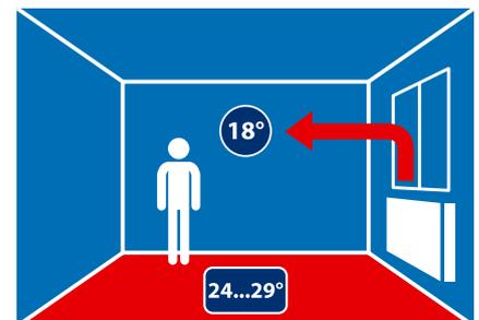
Accumulating heating system has to be controlled by special timer thermostat, to regulate the floor storage heating during low tariff periods and save energy. Thermostat is usually connected to an outdoor sensor, in order to constantly measure an outdoor temperature or weather conditions, and calculate amount of energy which has to be stored in floor. Alternatively a thermostat with a timer can also be used as a regulation unit.
