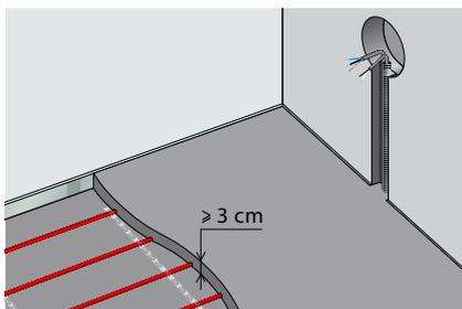
8. Check resistance and insulation values of cable and sensor. Apply concrete.
