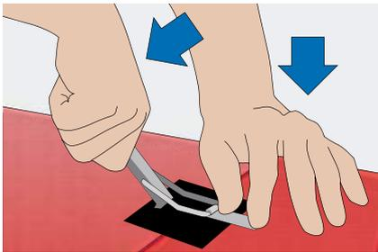
4. Push the elements/connectors tight together using the connector tool.
