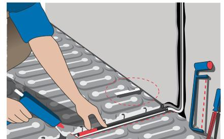
5. Cut out a hole for the warm/cold cable connection and the floor sensor conduit and file any sharp edges. Fix the conduit to the sub floor with glue or screws.
