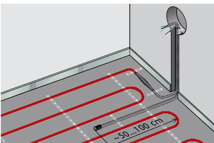
7. Install conduit pipe for floor sensor (must be sealed at the end installed in concrete). Check resistance of sensor before installing in pipe.
