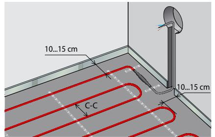
6. Check resistance and insulation values of cable. Install heating the heating cable: app. 10-15 cm from the walls. For comfort heating preferred C-C = 7,5 cm.
