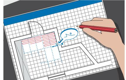
2. Draw a plan positioning cable, cold tail, floor sensor, thermostat and connection box, if any. Avoid all present and future objects fixed to the floor.
