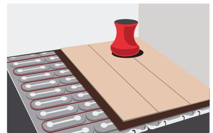
8. Install the floor finish at a room temperature of approximately 15 °C. Install a noise absorption mat and wooden floor, if desired.
