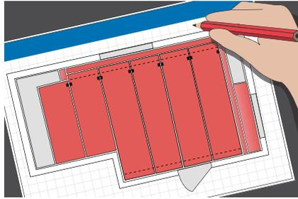
2. Recheck the layout, e.g. the placement of the control kit, floor sensors near the correct side of ECdry with male connector.
