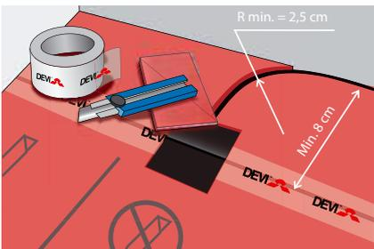
6. Cover the remaining part of the area with filler material. Cut out for supply and sensor cord and optionally extension cord.
