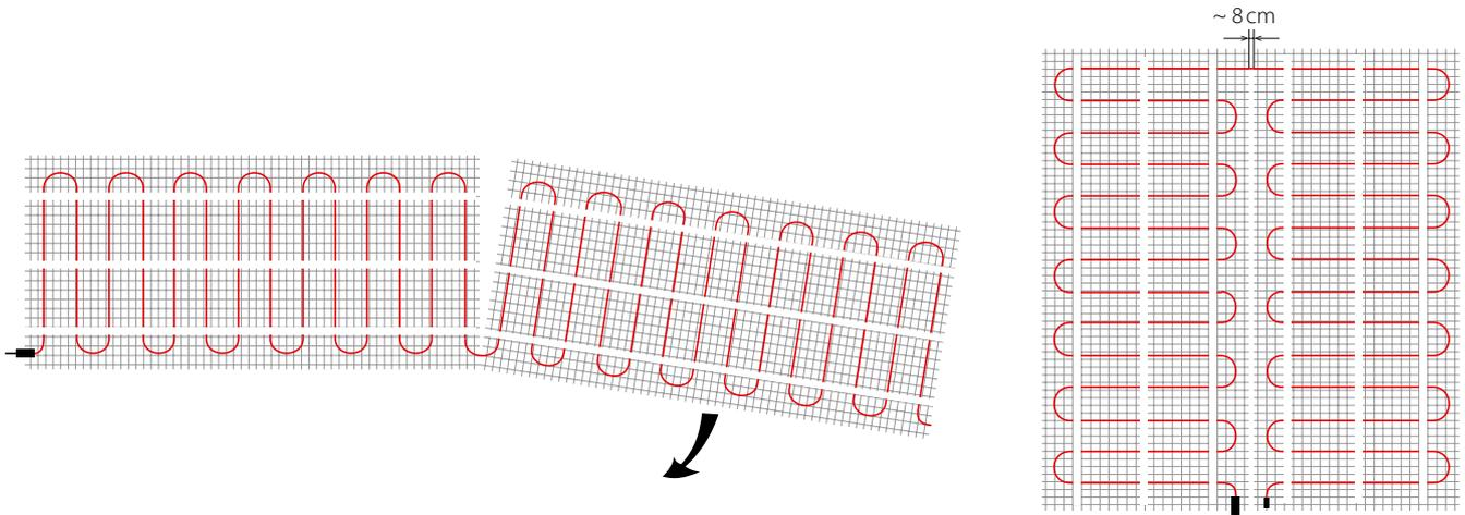
Fig. 9. The heating mats can be very easily adapted to the shape of the heated surface.
