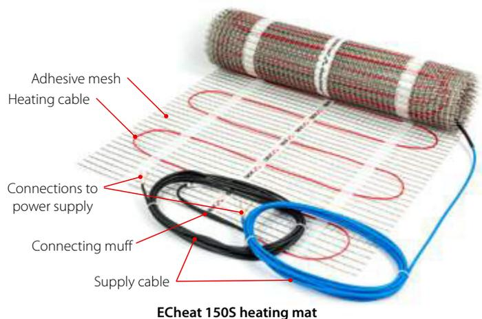
Center-to-center distance between mat's cable lines is usually 7,5 cm. It allows even distribution of heat on the floor surface avoiding cold zones between the cable lines.
