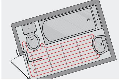
2. Draw a plan in order to position heated area, cable, cold tail, floor sensor, thermostat and connection box, if any.
