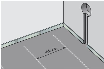
5. Fasten ECfast fitting bands in 50 cm distance (by nails, screws, dowels, hot melt glue etc.).
