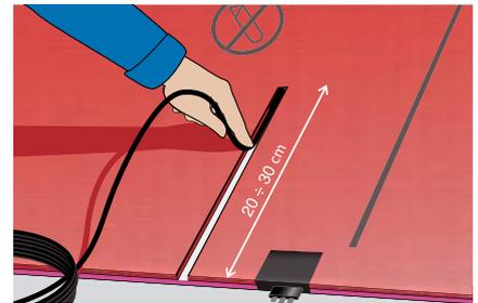
5. Rip off the pre-cut strip near supply cord connection and lay the sensor in the groove. Attach the included aluminum tape on top to fix the sensor cord.
