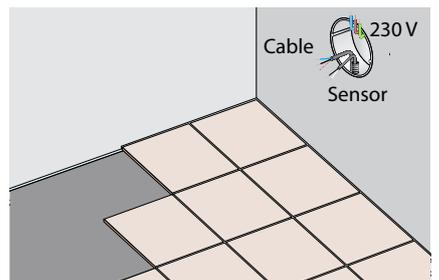
9. Check resistance and insulation values of cable and resistance of sensor. Install flooring and connect thermostat.
