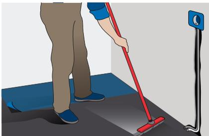
3. Cut out a wall groove and fix cable ducts and connection box. Clean the sub floor and lay out a vapor barrier or damp proof membrane (if required).
