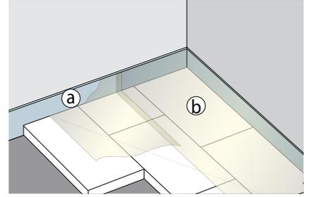
3. Install insulation: deformation tape (a), thermal insulation (b).
