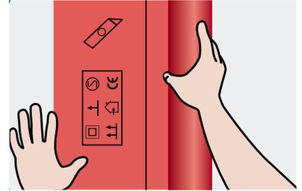
Make sure that the subfloor is reasonably level, firm and stable. Lay out a moisture barrier. Roll out the ECdry elements, the printed side of the elements must be visible.
