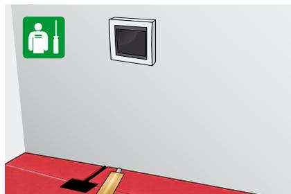
7. Check the insulation resistance of the heating elements. Install ECdry Touch Kit. Connect the cold tail, sensor and thermostat or plug the control into the socket.
