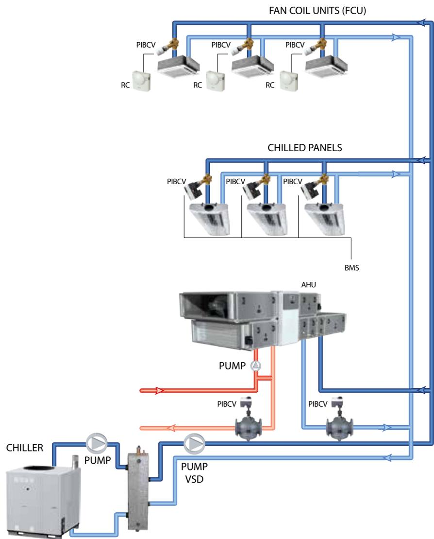
PIBCV – Pressure Independent Balancing Control Valves
