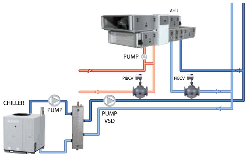
PIBCV – Pressure Independent Balancing Control Valve
