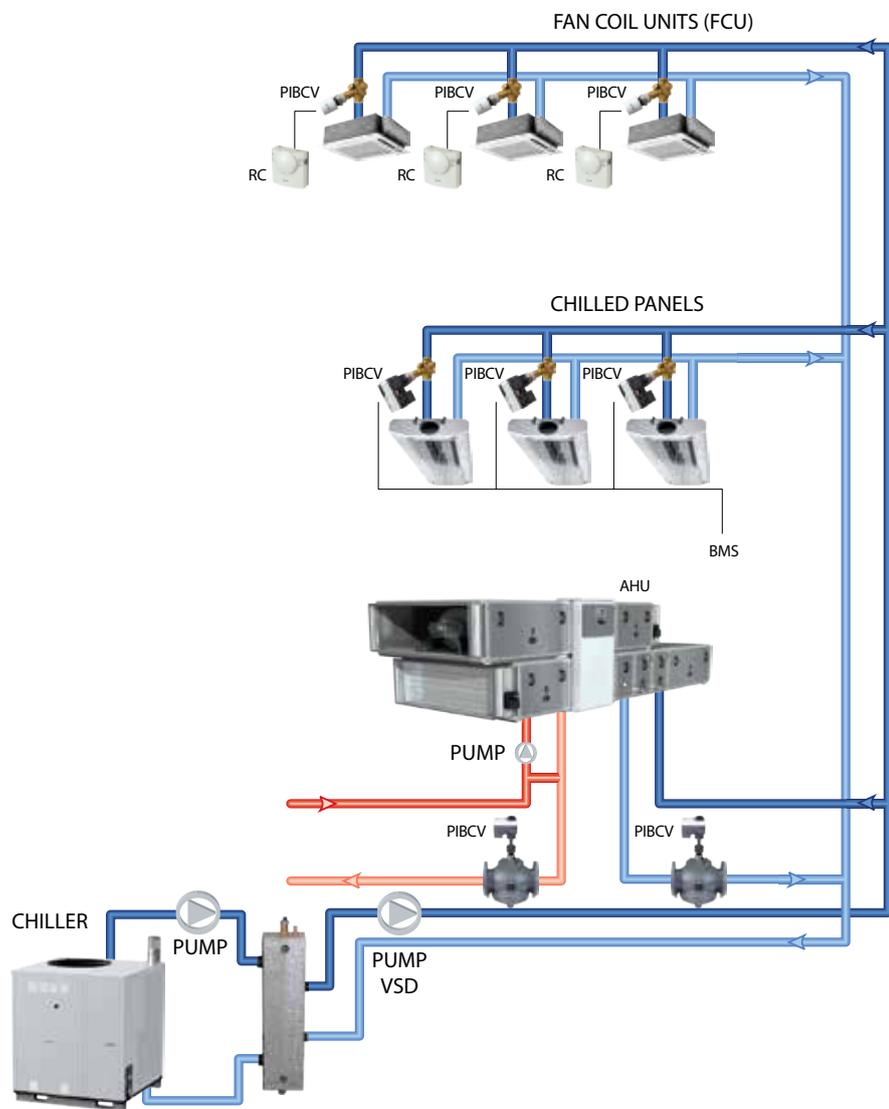
PIBCV – Pressure Independent Balancing Control Valves (as a flow limiter)
