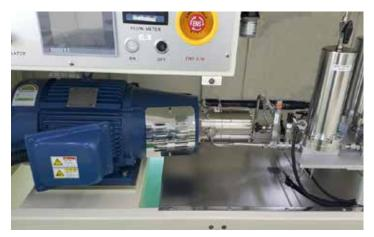
One of the Danfoss motor pump units with PAHT pump, installed at DMS.
